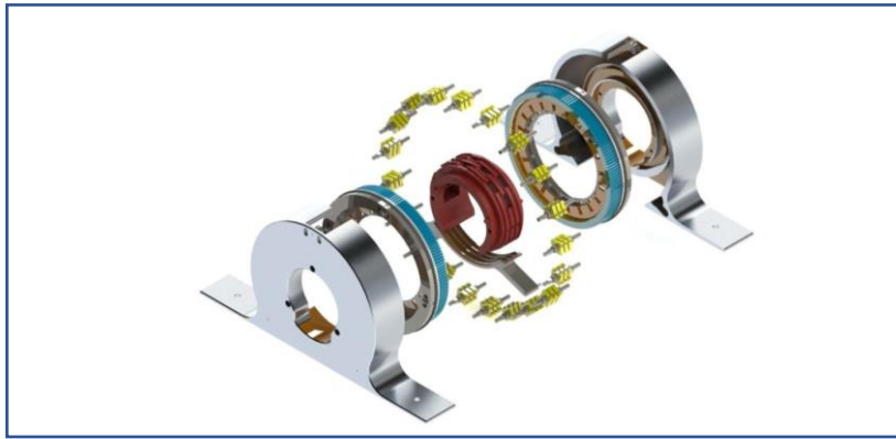
Exploded view of the main components to be assembled
