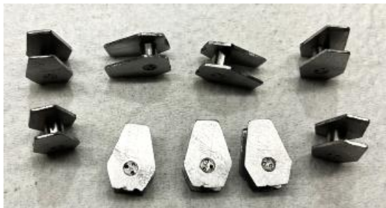
The nine actuators before coil-winding
