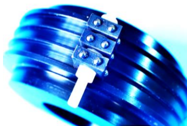
Three out of 60 Braille-cubes on axle
